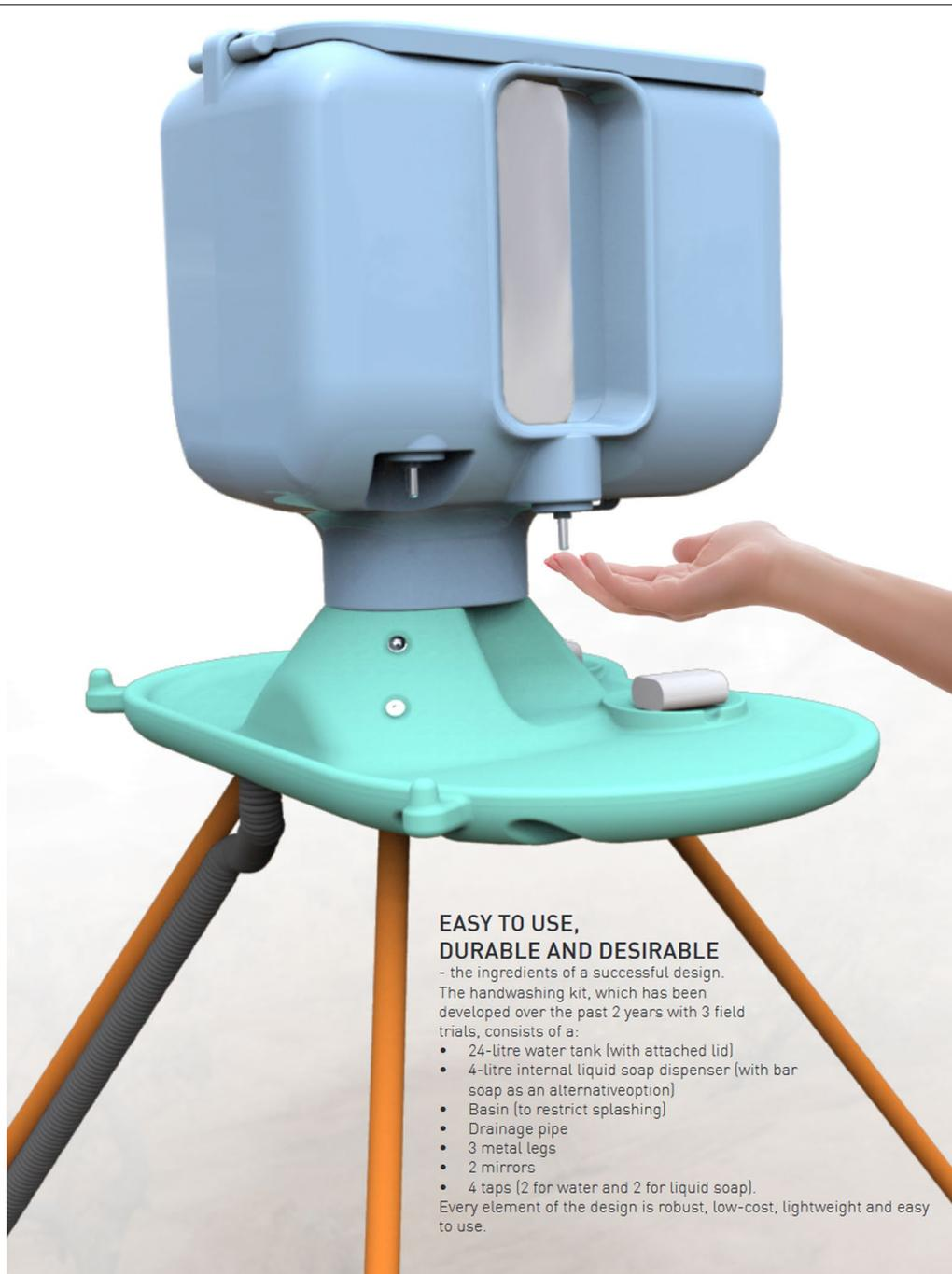
**Fig. 1** The Oxfam Handwashing Stand and a summary of its key features
